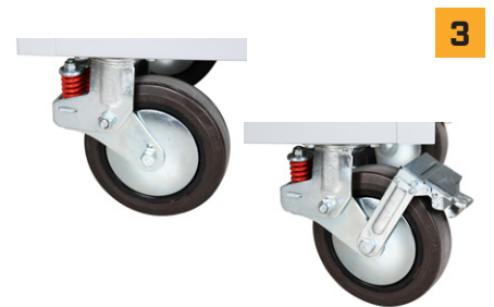
Spring mounted castor suspension, with locking device
