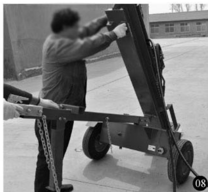
8. One person pulls out the bolt (on the drawbar, with spring inside) and presses the draw pole hard; the other person put the main body down slowly
