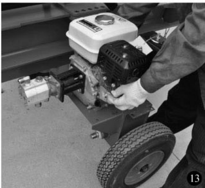
13. put the engine (with oil pump) at the correct position on the stand of machine.
