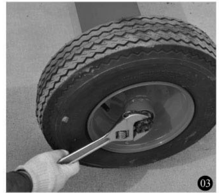
3. Fix the wheel with bearing on the axle of oil tank and fasten the nut with the wrench
